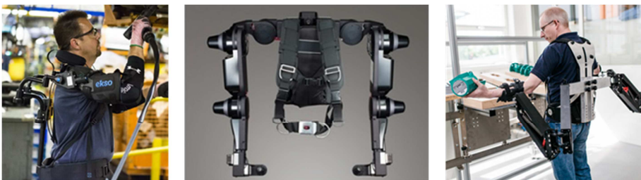
Figure 1. Typical examples of the wearable robots for upper extremities EksoVest, The Drive (Left), HEXAR-HL35, HEXAR SYSTEMS (Center), Passive Parallelogram Arms, Robo-Mate (Right)
