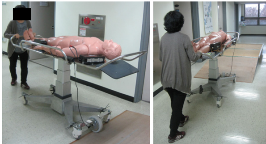
Figure 7. Measurement of muscle activities on the 10° sloped track
