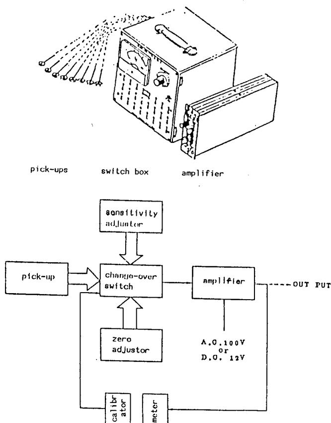
Fig. 1. Block Diagram of Elastic-Body Pressure Meter
