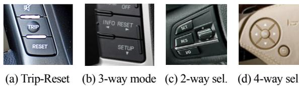
Figure 4. IVIS controller type in steering wheel
