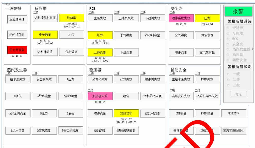
Figure 1. Alarm tile display example
