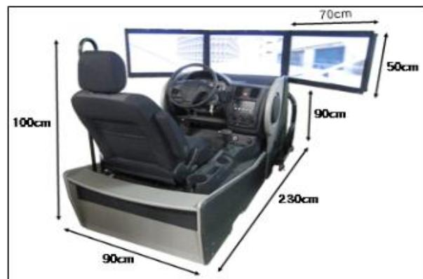
**Figure 1.** Graphic driving simulator
