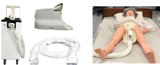
Figure 1. Excretion care robot (left) and elderly manikin (right)
