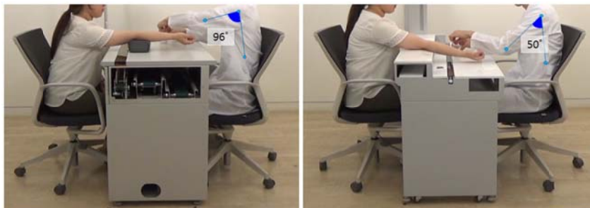
Figure 5. Comparisons of shoulder angles (left: original design vs. right: new design)
