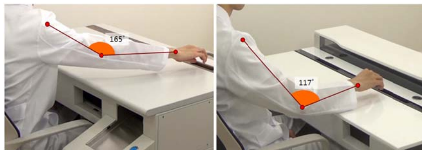
Figure 4. Comparisons of elbow angles (left: original design vs. right: new design)
