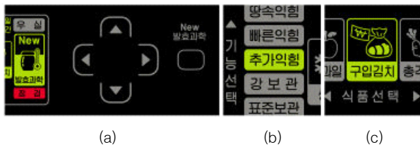
Figure 3. Control panel; (a) arrow keys, (b) mode selection keys, (c) food selection keys
