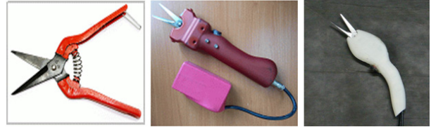
Figure 1. Hand-operated scissors, 1st prototype of Eletro-motion scissors and Completed Eletro-motion scissors
